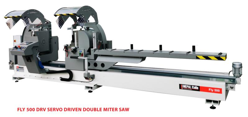
The FLY 500 DRV Double Miter Saw is a servo length positioned, double miter back cut saw with a fixed left head and numerically controlled positioning right head. Cut angles can be set by pneumatic actuators from 45°/90°/135° and intermediate angles utilize a manual set stop. The machine is equipped with a V8 touchscreen industrial CNC for easy operator interface.
